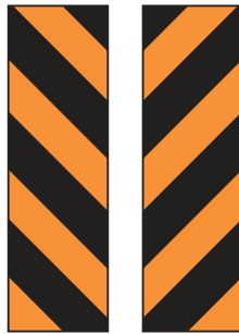
Hazard to left Hazard to right
