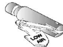
LOW PRESSURE WARNING
